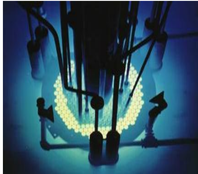
NSRR pulse reactor for RIA tests
